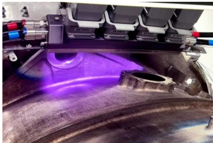
Figure 2 VCSEL laser in use on component part. Can see the different VCSEL modules arranged in an array at top of photo, and the light from the diodes on the part. The part is shown here which is due to be repaired. The bosses on the part will be re-welded or built up after damage. (Manufacturing Technology Centre, 2026)
