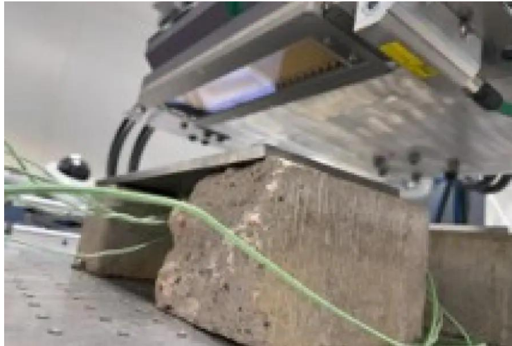
Figure 3: Image showing experimental set-up with VCSEL array at top of photo, and metal part with thermo-couples attached on heat-sink blocks at bottom of image. (Manufacturing Technology Centre, 2026)
